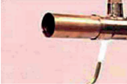
Cu to SS Tube Brazing
