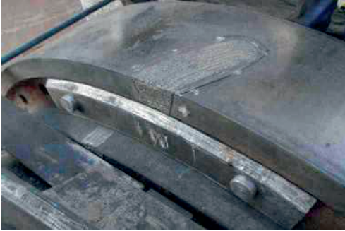
Kiln Tyre Crack Repair
