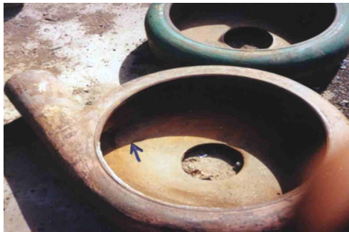
Slurry Pump Repair
